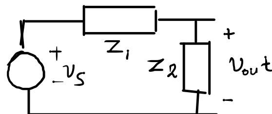
$$V_{out} = V_{in} \cdot \frac{Z_2}{Z_1 + Z_2} \quad (\text{Σιαρέζης τάξης}) \quad Z_1 = R, \quad Z_2 = \frac{1}{j\omega C}$$
