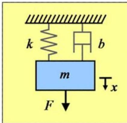
**Problem:** Model a 1 DOF mass-spring-damper system within the Simulink environment from first principles and using physical modeling tools.
