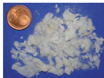
Fig. 1.2-15 A crop of 320 mg of caffeine isolated from green tea leaves according to the method described
