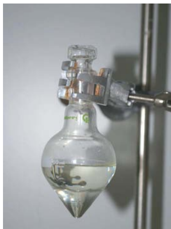
Fig. 2.2-4 A collection of a raw eugenol samples of a students' laboratory course was collected and distilled in vacuo. This 28 g sample was obtained starting from 400 g of cloves
