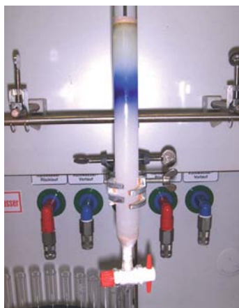
Fig. 2.3-4 Column chromatography of chamazulene
