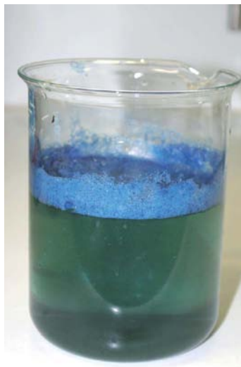
Fig. 3.4-12 Tiny indigo particles totaling not more than 3 mg are contained in the fluffy blue foam
