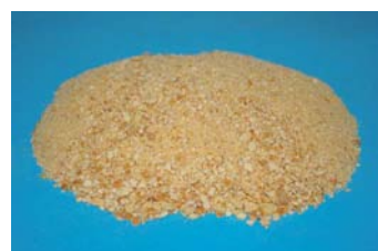
Fig. 4.4-6 Pile of dried, milled and pre-extracted mandarin orange peel prior to extraction with methanol
