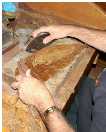
Figs. 1.1-2, -3 and -4 Leaves of tobacco plants are divided into five types: capa, ligero, capote, seco and volado. The composition of these types makes the secret of the cigar. Special attention is paid to the wrapper (capa), which is handled in a more humid state than the other leaves in a leather-like condition that makes it ductile
