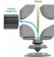
Quadrupole Ion Deflector turns ions 90 degrees
