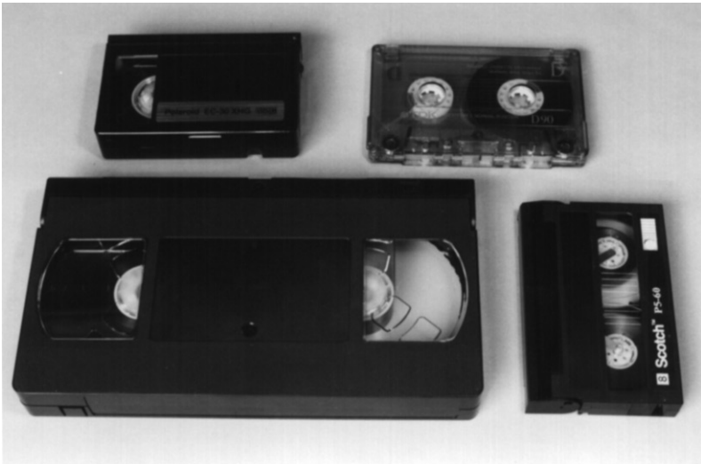
Figure 25.2 Cassette sizes compared. Clockwise from bottom right are Video-8, VHS, VHS-C and an audio Compact Cassette, shown here for size comparison
