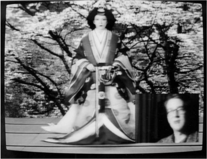
Figure 23.8 Picture-in-picture is one of the many effects afforded by a digital picture field store
