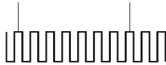
Figure 20.16 Combined FG and PG pulse train from the drum motor in Figure 20.15; the PG ‘needle’ pulses ride on top of the FG squarewave
