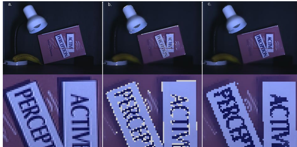
Fig. 18.12: Smoothing using dominant colors. (a): Original image not smoothed. (b): Smoothed image with transitional colors shown in light gray. (c): Smoothed image with transitional colors shown in the replacement dominant colors (if possible). Lower row shows detail images.
