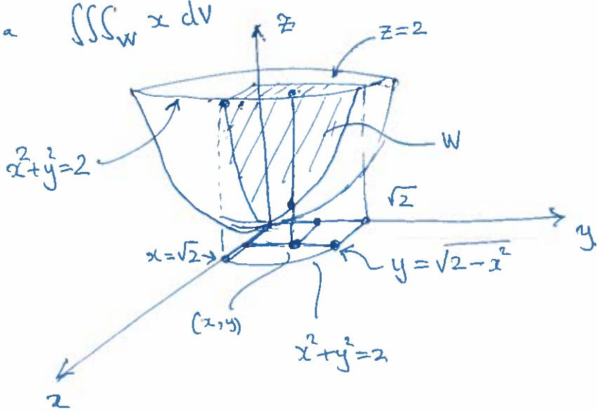
$$\iiint_W x \, dV = \int_{x=0}^{\sqrt{2}} \int_{y=0}^{\sqrt{2-x^2}} \int_{z=x^2+y^2}^2 x \, dz \, dy \, dx$$
