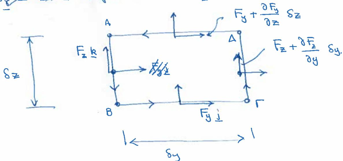
$$\begin{aligned} \int_S \underline{F} \cdot d\underline{s} &\approx -F_z \delta_z + F_y \delta_y + \left( F_x + \frac{\partial F_x}{\partial z} \delta_z \right) \delta_z \\ &\quad - \left( F_x + \frac{\partial F_x}{\partial y} \delta_y \right) \delta_y. \end{aligned}$$
