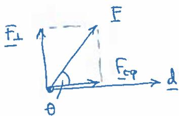
$$W = \underline{F} \cdot \underline{d} = \|\underline{F}\| \cdot \|\underline{d}\| \cos \theta = (\|\underline{F}\| \cos \theta) \|\underline{d}\| = \|F_{\text{eq}}\| \cdot \|\underline{d}\|$$
