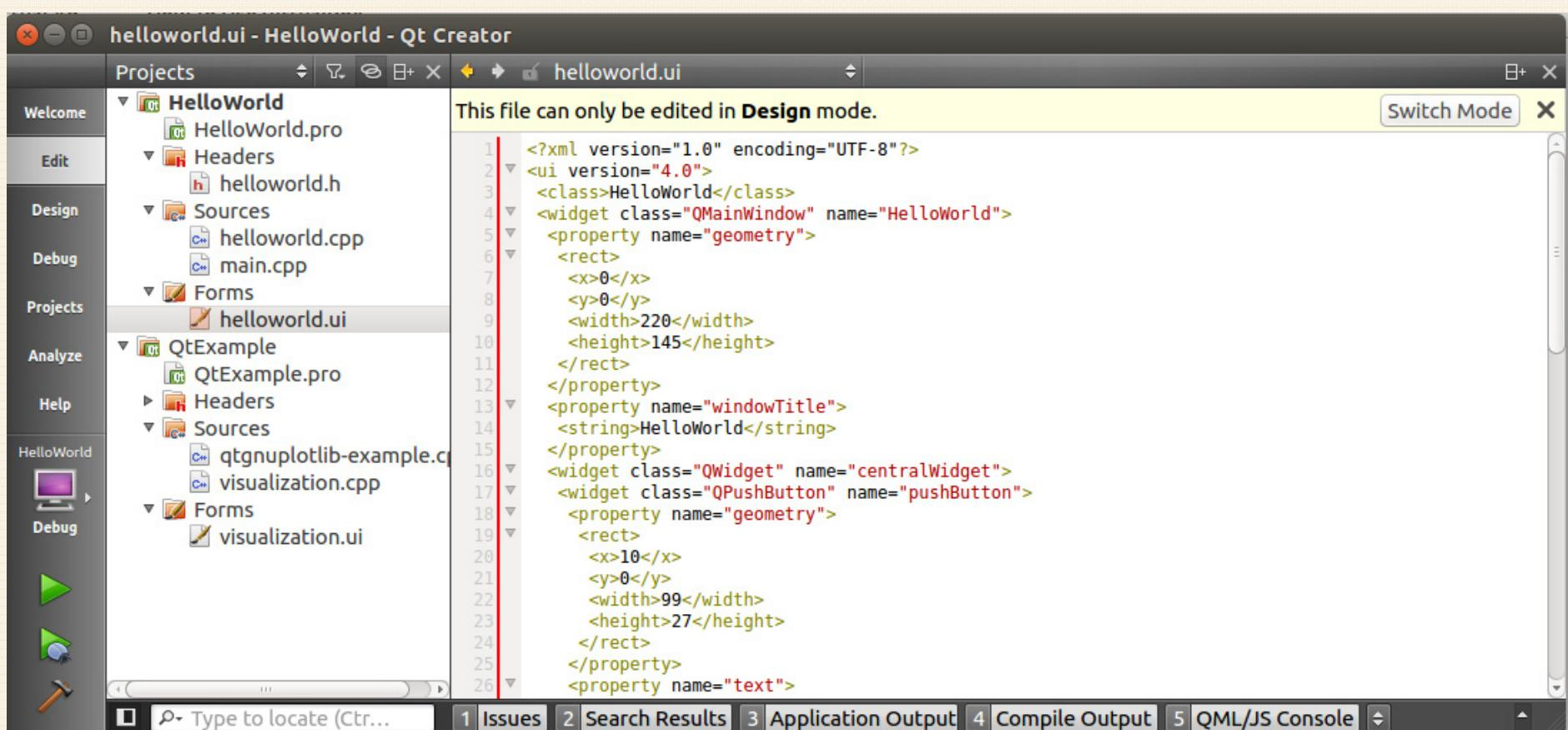
The screenshot shows the Qt Creator interface with the project "helloworld" selected. The left sidebar shows the project structure with files like HelloWorld.pro, helloworld.h, helloworld.cpp, main.cpp, and helloworld.ui. The main editor area displays the XML code for the UI file:
