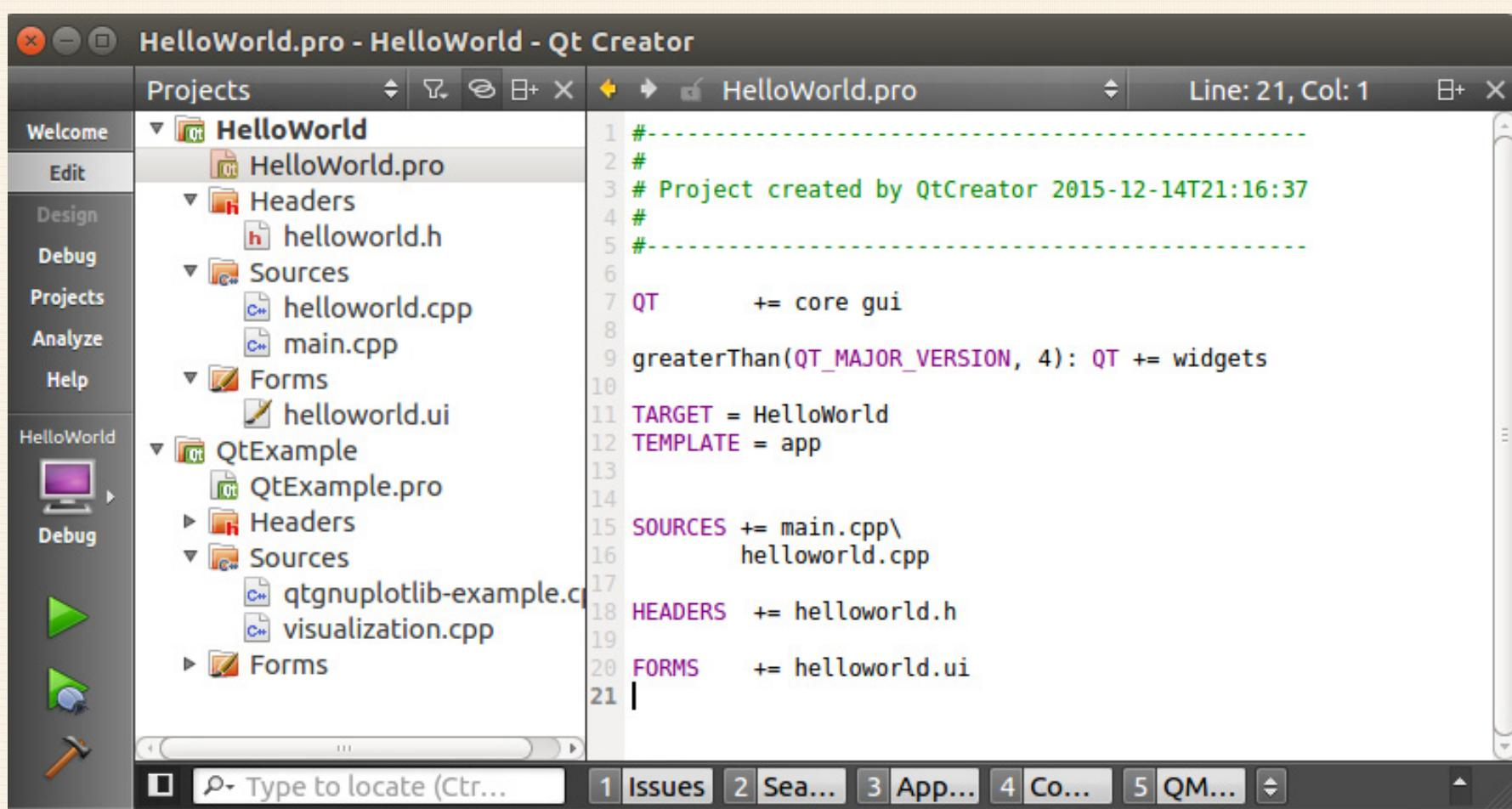
The screenshot shows the Qt Creator interface with the project "HelloWorld.pro" selected. The left sidebar displays project navigation, and the bottom bar includes icons for file operations and a search bar. The main area shows the project structure and its corresponding .pro file content.
