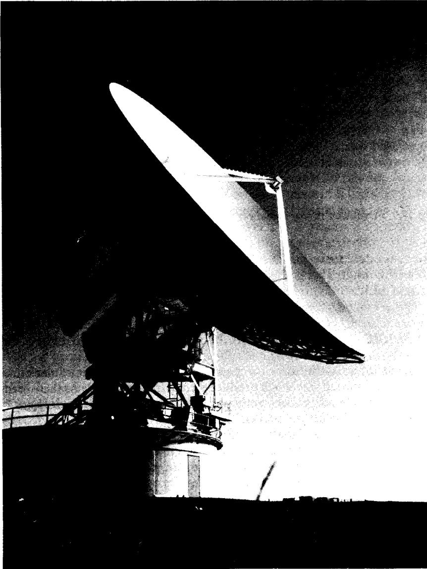
Fig. 14.8 Photograph of antenna and beam waveguide feed.
