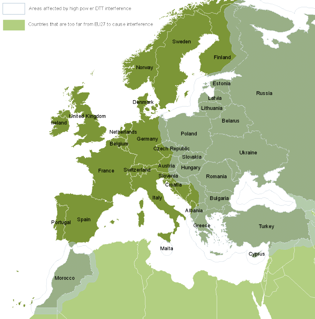
Figure 13.3: Assumption of regions in which harmful interference is caused by countries using the 790–862MHz sub-band for high-power DTT (in the Reference Scenario) [Source: Analysys Mason, DotEcon and Hogan & Hartson, 2009]
