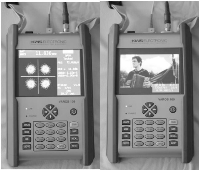
Fig. 15.9. Measurements on a satellite antenna system using an antenna test receiver (KWS VAROS 109). Left side: important measurement parameter (level, MER, BER) and constellation diagram. Right side: decoded video signal; the equipment also includes an LNB interface with optical IF output.
