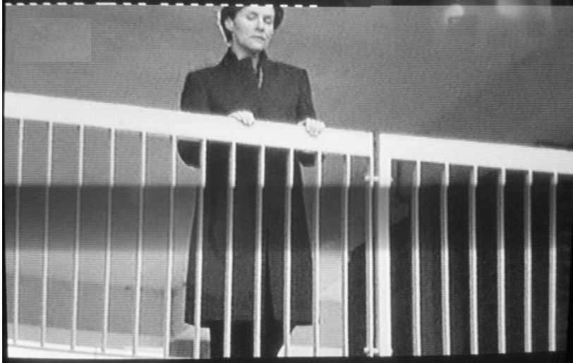
Fig. 9.11. Visible WSS signal on a TV screen (top, left-hand side)
