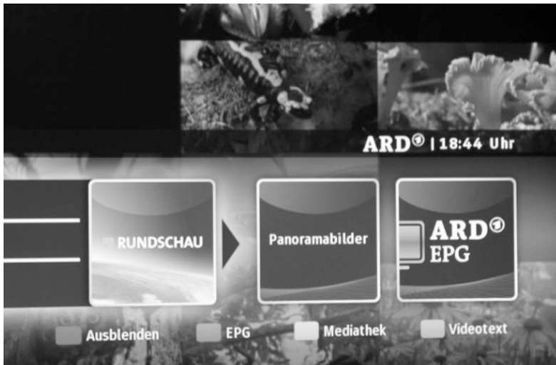
Fig. 44.4. Example of HbbTV services (access via color function keys on the TV remote control)
