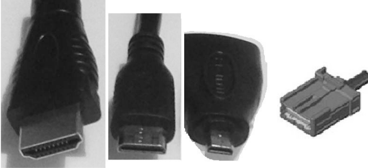
Fig. 10.16. HDMI plug types (from left): type A ("standard"), type C ("mini"), type D ("micro") and type E ("automotive")
