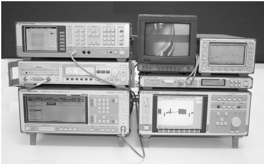
Fig. 18.20. Constellation analysis on a DVB-C signal from a test transmitter (Rohde&Schwarz SFQ, bottom left) using a test transmitter (Rohde&Schwarz EFA, top left): An MPEG-2 generator (Rohde&Schwarz DVRG, center left) supplies an MPEG-2 transport stream with test contents which is fed into the test transmitter. The DVB-C receiver EFA displays the DVB-C Signal back into the MPEG-2 transport stream which can then be decoded with an MPEG-2 test decoder (Rohde&Schwarz DVMD, center right). The picture also shows the video analyzer VSA (bottom right), the TV monitor (top center) and a “601” analyzer VCA (top right).
