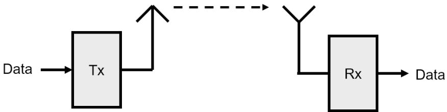
Fig. 37.35. SISO = Single Input – Single Output
