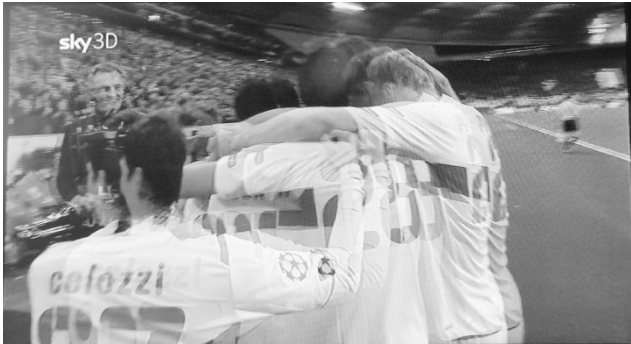
Fig. 43.12. Display in 3D mode, without shutter glasses (Sky 3D), disparity (left-/right shift) well visible
