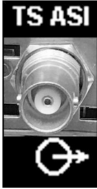
Fig. 10.9. TS-ASI connector (75 Ohms, BNC)
