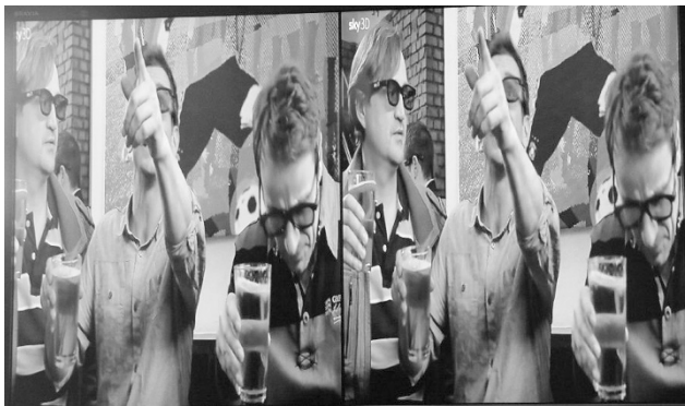
Fig. 43.11. Practical example for side by side transmission (Sky 3D), display in normal mode
