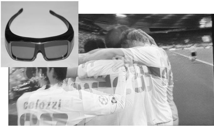
Fig. 43.1. 3D-picture shown on a flat screen without using 3D glasses; top left 3D shutter glasses which are necessary to generate the 3D effect for the eyes.
