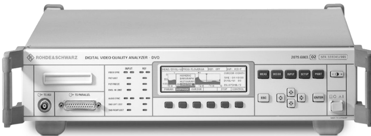
Fig. 12.10. Digital video quality analyzer, Rohde&Schwarz [DVQ] for MPEG-2-video-based video coding quality measurements
