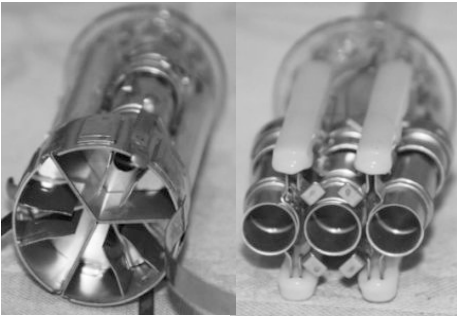
Fig. 34.6. Electron beam gun of a delta-type (left) and in-line-type (right) shadow mask tube
