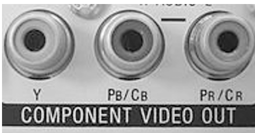
Fig. 10.1. RCA sockets, for component video signals in this example
