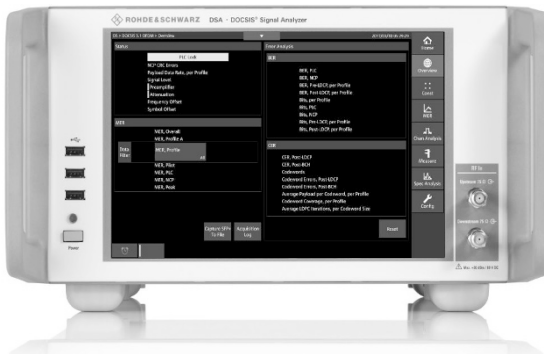
Fig. 18.23. DOCSIS Analyzer DSA, Rohde&Schwarz, including a DVB-C Analyzer
