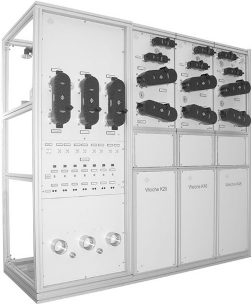
Fig. 46.50. Example for an antenna combiner for 3 channels (5 kW each); each combiner module can be bridged, each combiner input can be connected to a dummy antenna; manufactured by Spinner [SPINNER]
