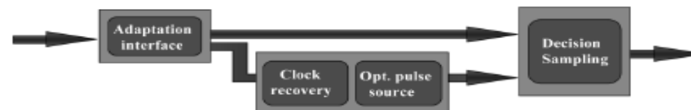
Fig. 2. Generic layout of a 3R regenerator using nonlinear gates.
