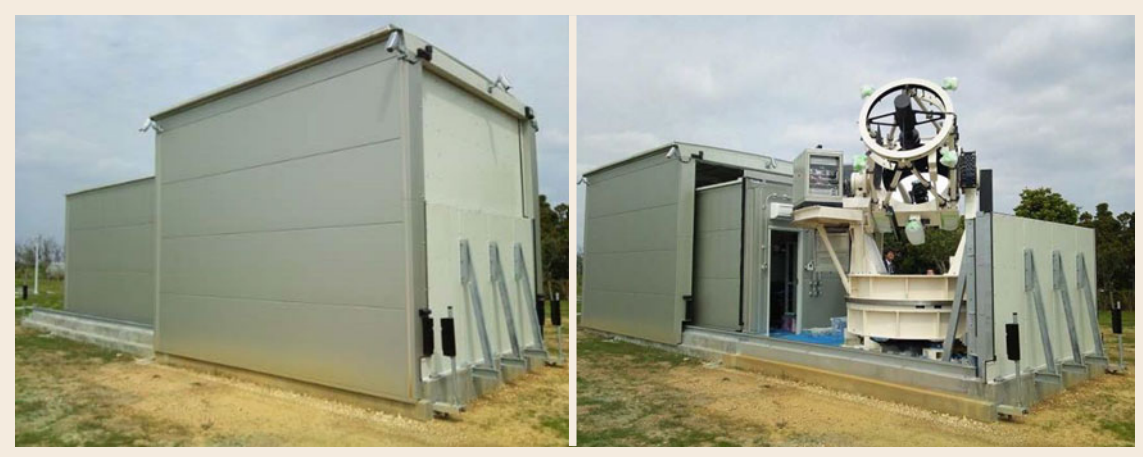
Fig. 34.26 Compact and remotely controlled 1 m OGS in Okinawa (Japan) built by NICT
