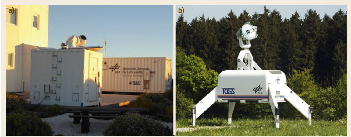
Fig. 34.35a,b DLR transportable adaptive optics ground station (a). DLR transportable optical ground station (b)
