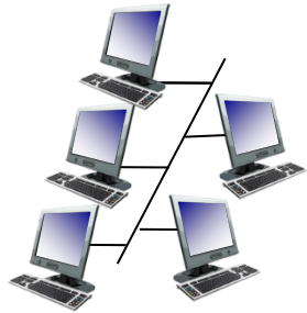
shared wire (e.g., cabled Ethernet)
