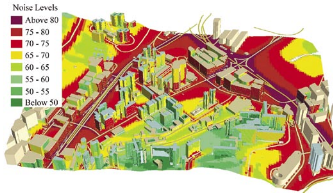
Figure 2. Noise model in 3D for impact assessment of road traffic noise (Db) in Kwai Chung new town, Hong Kong. Noise levels shown in the model are for indicative purpose and do not relate to actual traffic noise levels on site (Source: Environmental Protection Department, Hong Kong SAR).
