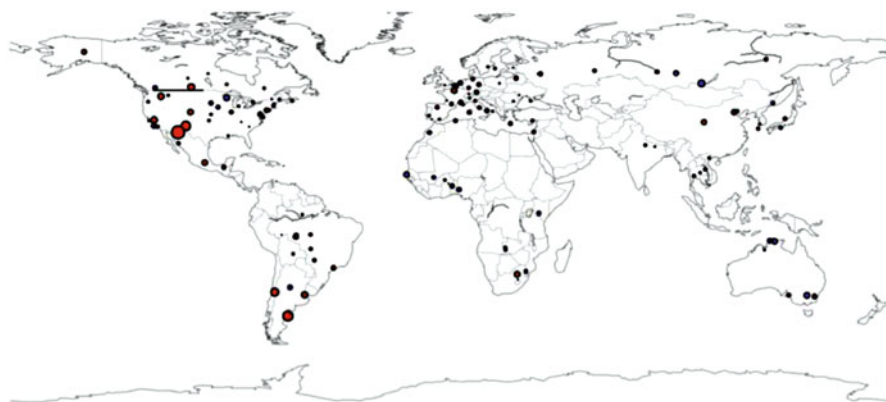
Fig. 7 MODIS bias with respect to AERONET. Computed as a regression with intercept at the origin. Red indicates that MODIS is higher; blue indicates that AERONET is higher. The size of the circle is proportional to the slope of the regression for slope > 1 (where MODIS is higher) and to the inverse of the slope for slope < 1
