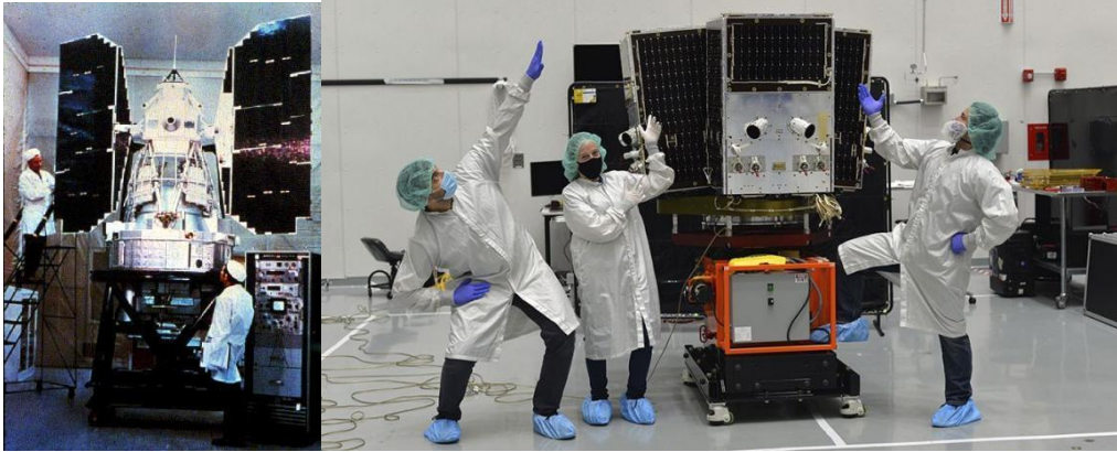
Figure 3 Satellite Size Comparison: Landsat-1 (Left) vs. Skysat (Right)
