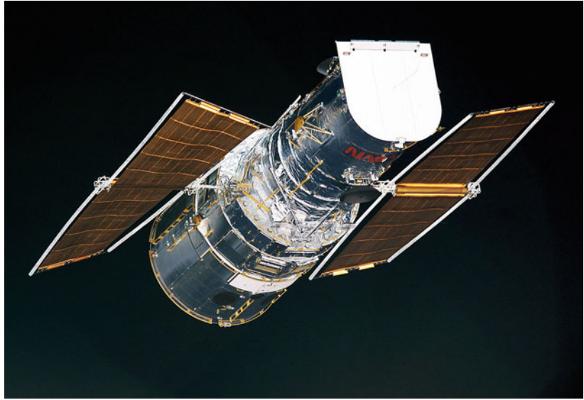
The Hubble Space Telescope receives power from solar cells (NASA).
