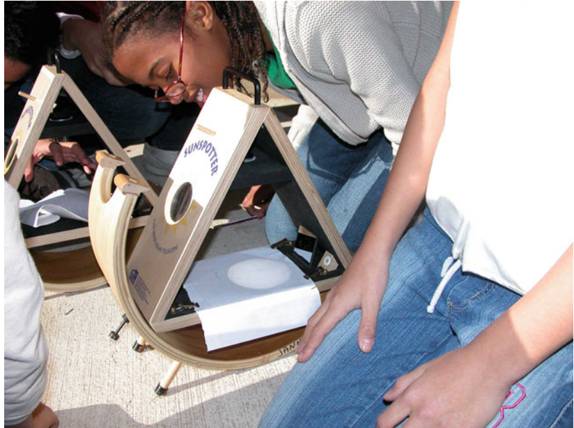
A sunspotter is a simple and practical instrument that makes it easy to observe the Sun safely (NASA).
