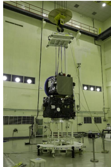
Proba-3 Satellites successfully stacked ahead of hydrazine fueling
