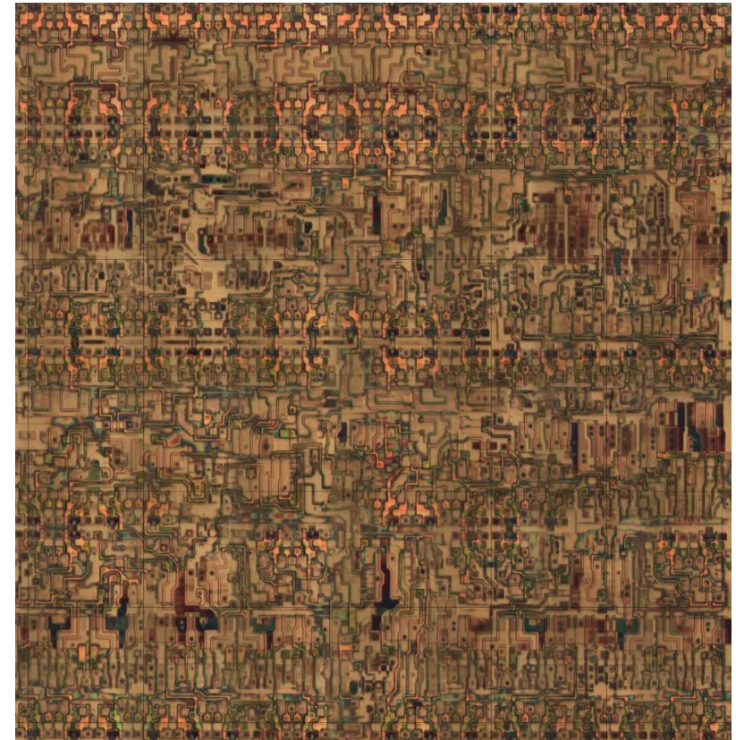
Die closeup showing circuitry for one of the 64 tiles in XC2064 FPGA
