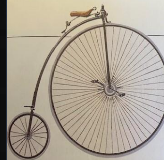
▲ The first bicycles were uncomfortable and dangerous. This 'penny-farthing' of 1883 had solid tyres and no brakes.
