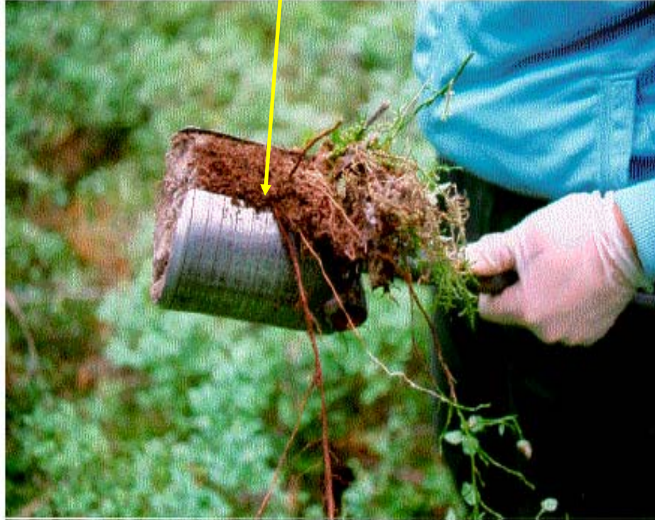
Fig. 8a. Humus sampling in Finland using cylindrical sampler. (Photographs: Timo Tarvainen).
