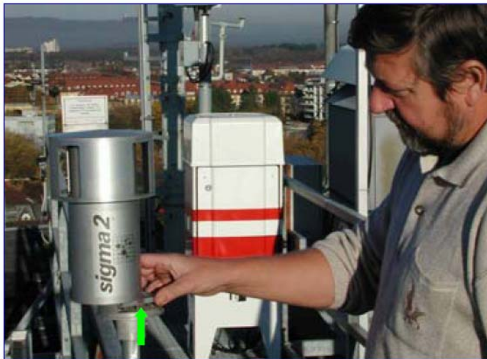
FIGURE 1. Schematic and photograph of PUF disk passive air sampler.
