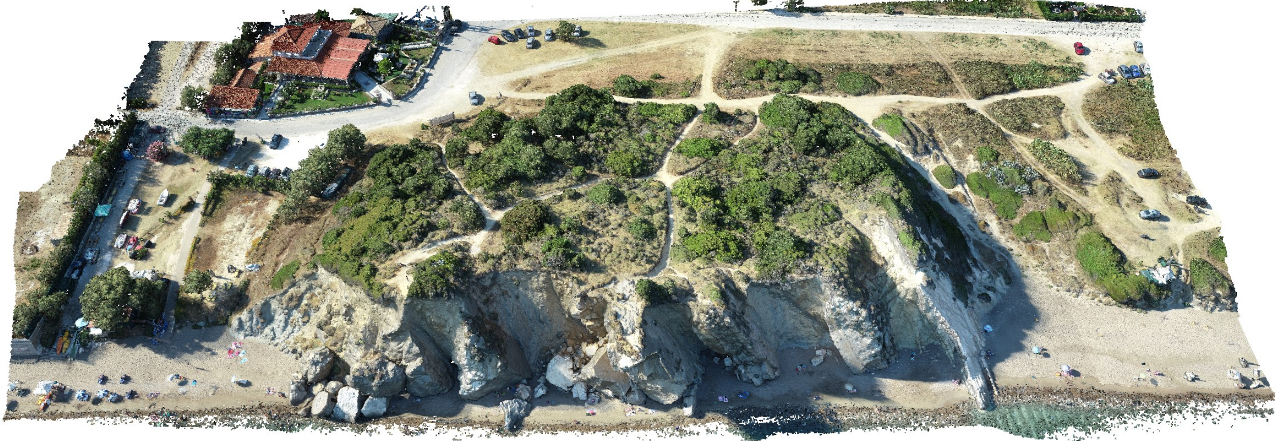
UAS Structure from Motion Photogrammetric processing
