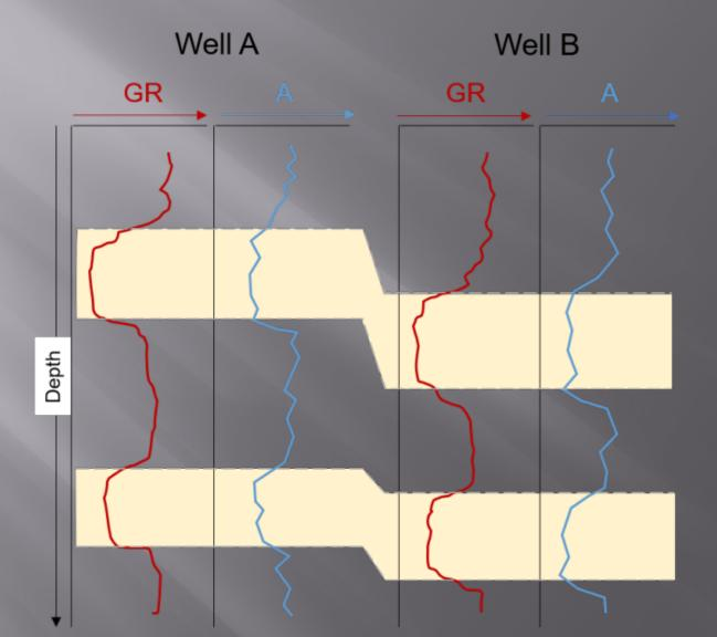
Correlation between well A and well B based on GR and lithology depending element (A).
