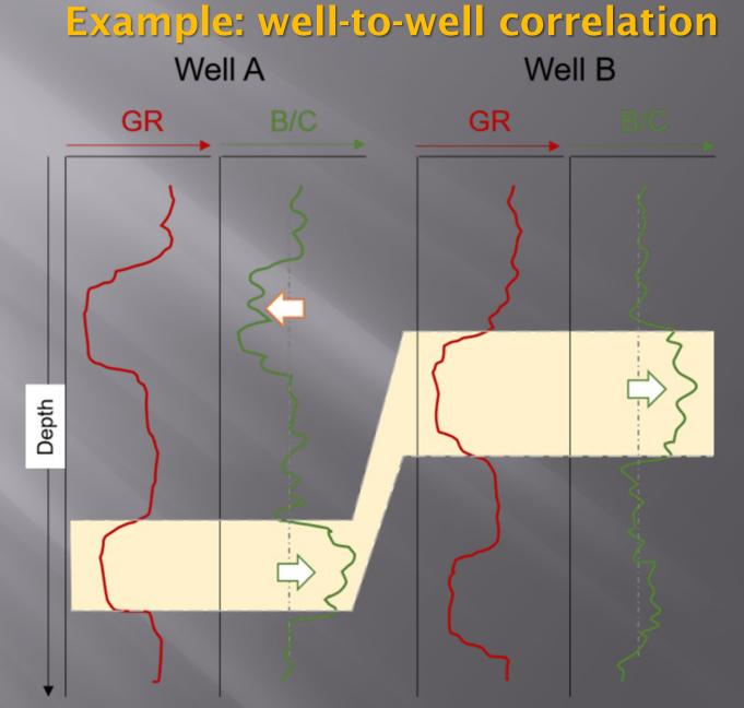
Correlation between well A and well B based on lithology independent element/element ratio (B/C).
