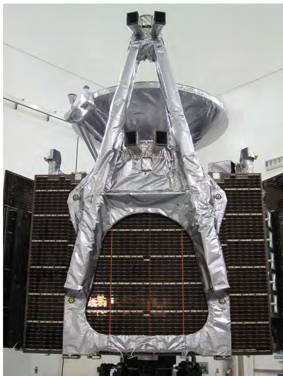
The Magnetometer experiment for the Juno orbiter for Juno can be seen here on the end of a boom. The spacecraft uses two fluxgate magnetometers. (see also Magnetometer (Juno) )
