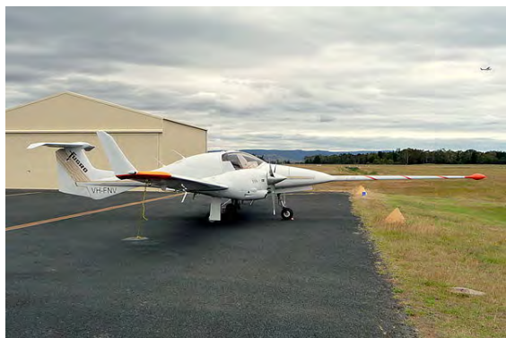
A Diamond DA42 light aircraft, modified for aerial survey with a nose-mounted boom containing a magnetometer at its tip
