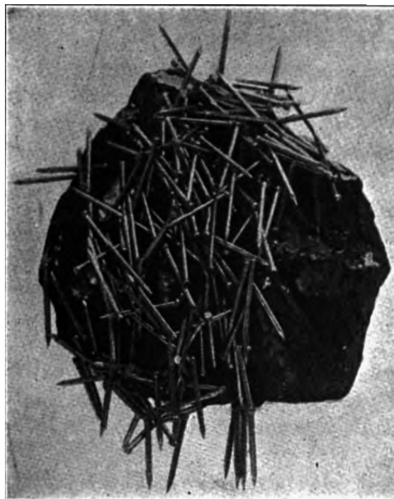
Lodestone, a natural magnet, attracting iron nails. Ancient humans discovered the property of magnetism from lodestone.
