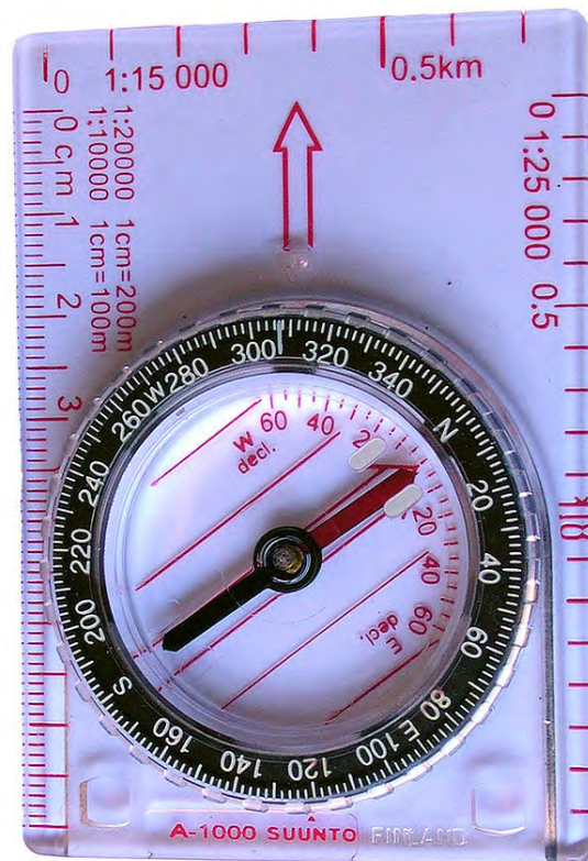
Adjustable compass set to a declination of 0° and a bearing of 307°
