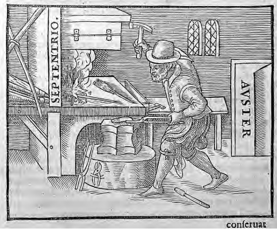
An illustration from Gilbert's 1600 De Magnete showing one of the earliest methods of making a magnet. A blacksmith holds a piece of red-hot iron in a north-south direction and hammers it as it cools. The magnetic field of the Earth aligns the domains, leaving the iron a weak magnet.
