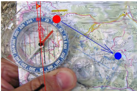
Turning the compass scale on the map (D – the local magnetic declination)
