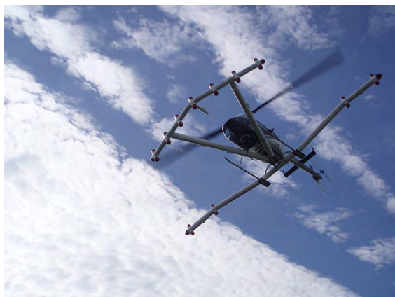
This helicopter is equipped with a magnetometer array. It flies six feet above ground at speeds of 30 to 40 mph.
