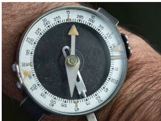
Wrist compass of the Soviet Army with counterclockwise double graduation: 60° (like a watch) and 360°
