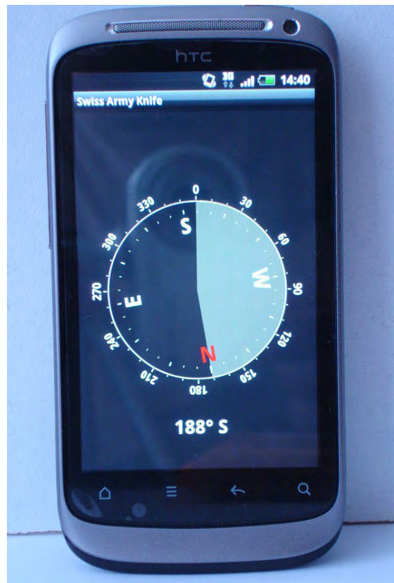
A smartphone that can be used as a compass because of the magnetometer inside.
