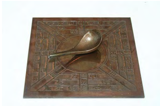
A reconstruction of an early Chinese compass. A spoon made of lodestone, its handle pointing south, was mounted on a brass plate with astrological symbols.* [1]
