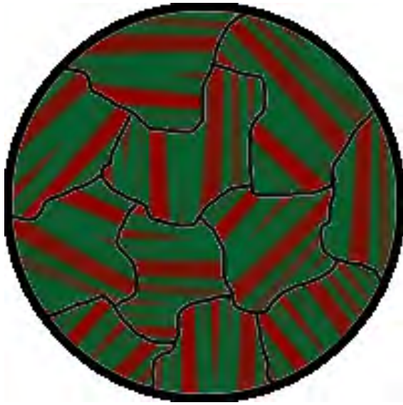
Kerr micrograph of metal surface showing magnetic domains, with red and green stripes denoting opposite magnetization directions.
