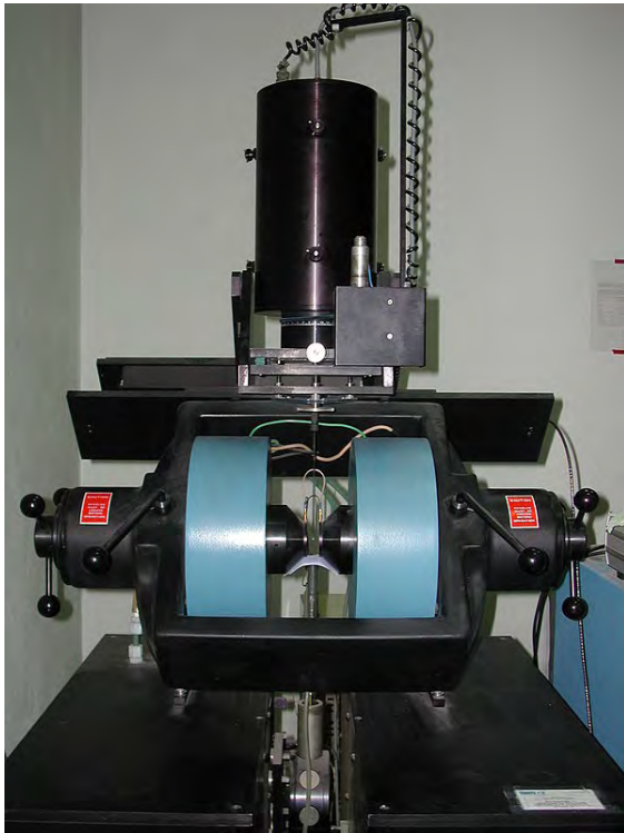
A vibrating sample magnetometer, a widely used tool for measuring magnetic hysteresis.
