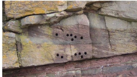
Cluster of corings in cross bedded sandstone, Late Devonian, Portishead, Somerset. Photo. Dave Evans, Natural England.
