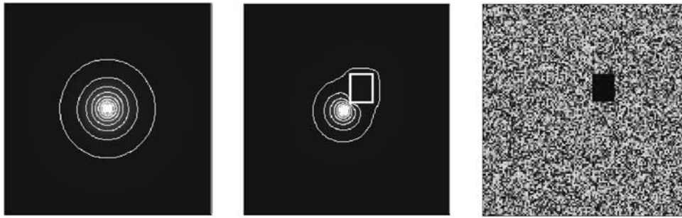
Figure 10. (left) FEM solution of the diffusion equation for a point source. Contours give regions of same pore pressures and are circles around the source for an isotropic homogeneous diffusivity field. (middle) A diffusivity heterogeneity (rectangle, with a higher diffusivity than the background) which causes a distortion in the pressure distribution (here a faster pressure increase due to the high-diffusivity patch). (right) Criticality field with randomly distributed criticality values in the background and a highly critical patch (dark rectangle). Dark cells correspond to more critical regions, meaning that lower pressure changes can trigger earthquakes. So, bright cells represent more stable regions.
