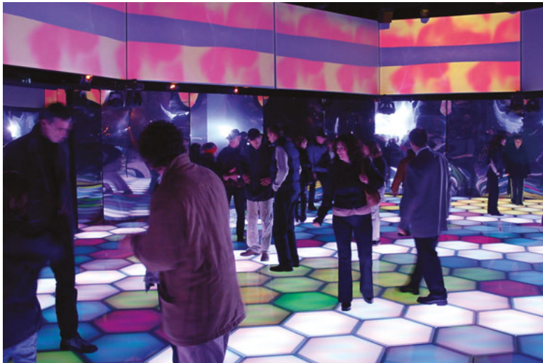
Figure 16.3 The ADA main space (180 m 2 ) engages with its visitors through interactive multimodal compositions. The hexagonal floor tiles are pressure sensitive and display colored patterns dependent on ADA's behavior modes and visitor interactions. The walls are made of semitransparent mirrors, which permit visitors in the outer corridor to view what happens inside ADA. Above the mirrors, a circular projection screen displays real-time animated graphics which, similar to the music, represent Ada's current behavior and emotional state. ADA was operational from May until October, 2002, and was visited by over 500,000 people.
