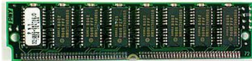
SIMM: Single In-line Memory Module (32bit data path)
