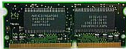
SODIMM: Small Outline Dual In-line Memory Module (notebooks)
