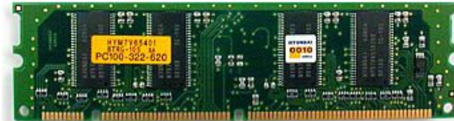
DIMM: Dual In-line Memory Module (64 bit data path)
