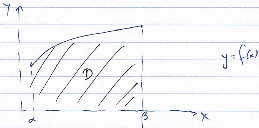
$$A(D) = \int_D dxdy = \int_{\alpha}^{\beta} \left\{ \int_0^{f(x)} dy \right\} dx = \int_{\alpha}^{\beta} f(x) dx$$
