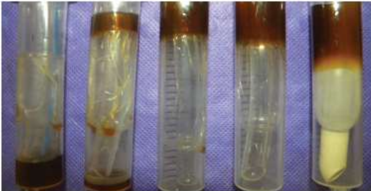
Figure 2. Photograph of various bench tested tracheal tubes of different designs showing the internal channels created and the leak of liquid material past the cuff. Tube cuffs A and B are made from polyvinyl chloride, and cuffs C and D with thin polyurethane (C has an elongated cylindrical shape and D is a tapered cuff design). Tube E is the LoTrach™ ET tube. (Photograph courtesy of Dr Peter Young, Kings Lynn, UK.)
