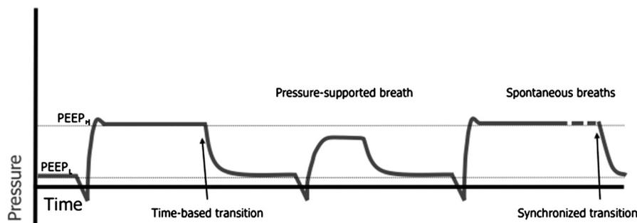
**Fig. 7.** Biphasic ventilation mode. After selecting biphasic ventilation mode, 2 different levels of PEEP ( $PEEP_L$  and  $PEEP_H$ ) are chosen. Spontaneous breaths may be taken during the time when  $PEEP_H$  is applied (dashed lines); pressure-supported breaths are given during the time when  $PEEP_L$  is applied. The transition between the 2 levels of PEEP may be after a set time interval or synchronized with patient effort.
