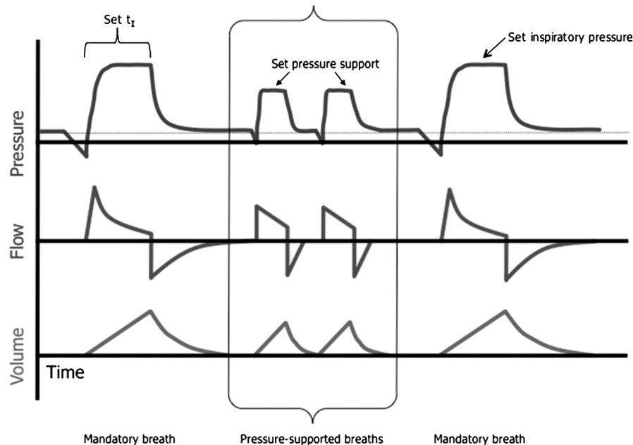
**Fig. 4.** Synchronized intermittent mandatory ventilation plus pressure support ventilation (SIMV + PSV) in PC mode. The first and last breath tracings are identical to those seen in standard PC mode: patient- or time-triggered, pressure-limited, and time-cycled. However, spontaneous breaths (bracketed) are pressure-supported and thus patient-triggered, pressure-limited, and flow-cycled.  $t_i$ , inspiratory time.
