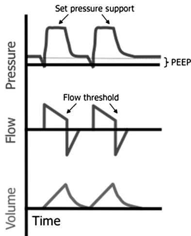
**Fig. 3.** Pressure support ventilation mode. After patient effort triggers the ventilator, a set pressure is applied until flow, which is decelerating, reaches a threshold level. The ventilator then cycles off, and the patient passively or actively exhales. Thus, PSV mode is patient-triggered, pressure-limited, and flow-cycled.
