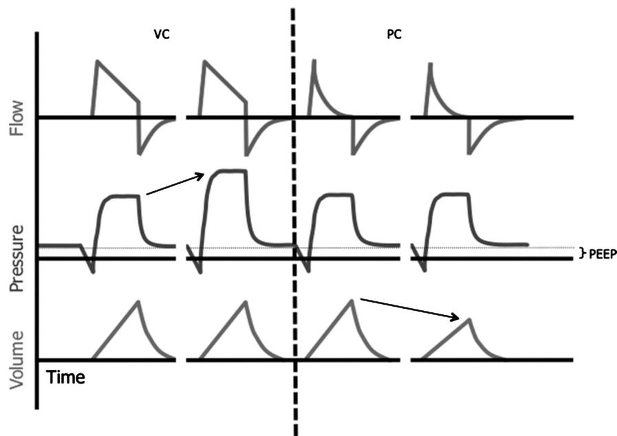
**Fig. 10.** Responses to changes in respiratory system compliance. When faced with a decrease in respiratory system compliance, the ventilator in a volume-controlled mode will continue to deliver a set tidal volume at the expense of increased pressure (first and second tracings). Pressure modes such as PC maintain a set inspiratory pressure, which results in a decreased tidal volume as compliance decreases (third and fourth tracings).
