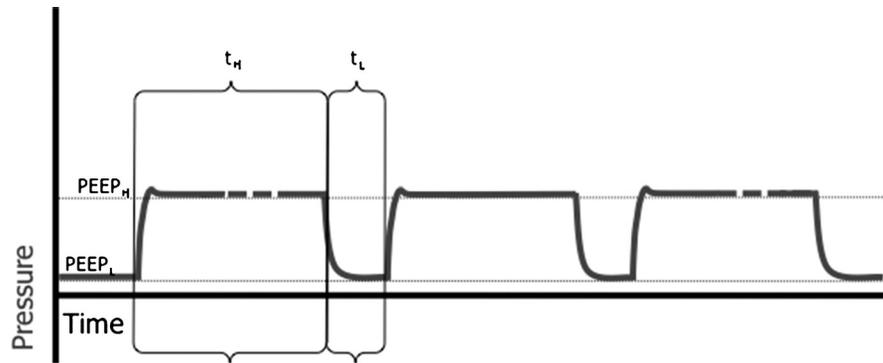
**Fig. 6.** Airway pressure release ventilation mode is an inverse ratio mode of mechanical ventilation in which the time spent at high lung pressure ( $PEEP_H$ ) exceeds that spent at low lung pressure ( $PEEP_L$ ). Unsupported spontaneous breathing (dashed lines) is allowed and occurs mainly during  $t_H$  because of the short period of time spent at  $t_L$ .
