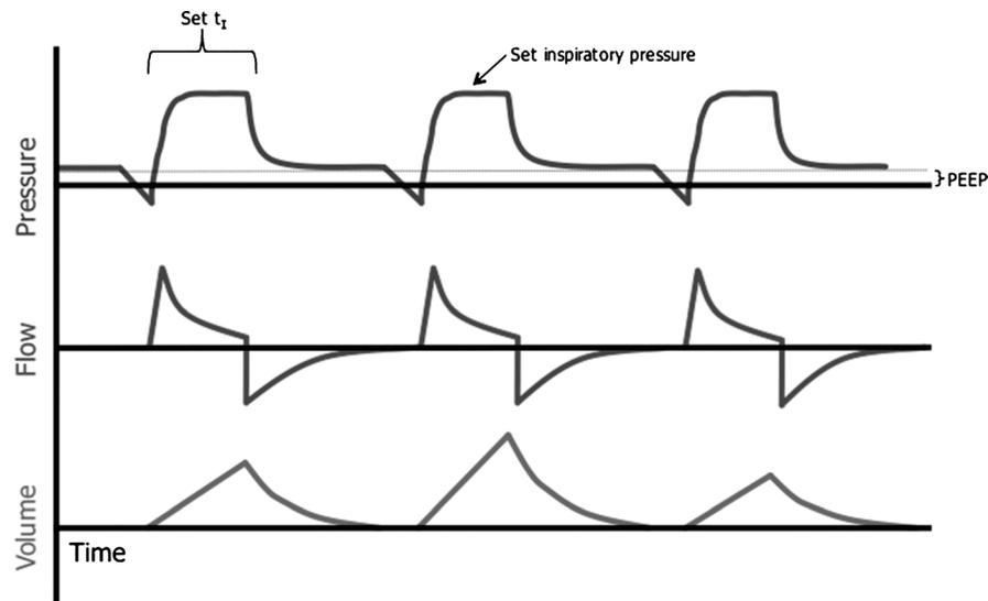
**Fig. 1.** Pressure control ventilation (PC) mode. In contrast to volume-controlled modes of mechanical ventilation, the ventilator in PC mode applies a set inspiratory pressure over a set inspiratory time. Thus, PC mode is patient- or time-triggered, pressure-limited, and time-cycled. Tidal volume is variable and depends in part on patient mechanics.  $t_i$ , inspiratory time.
