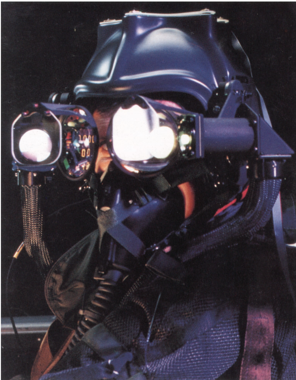
The CAE-Link Helmet Mounted Display (HMD), an early 1990s model for use in aviation instruction, is shown here; it enables bright, high-resolution, full-color computer-generated imagery to be projected over an unlimited field of vision. HMDs are specifically designed to duplicate the operation and performance of the human eye. By monitoring the direction the wearer is looking, imagery is generated that covers the line of sight. HMD displays can easily be combined with other sensor simulations such as Forward Looking Infrared (FLIR) devices, for example. See also pages 1037 and 1041. (Courtesy, CAE-Link Corp.)
