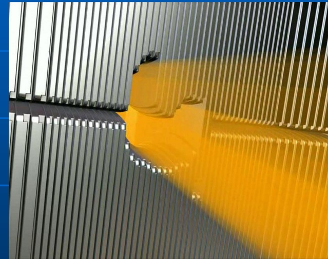
A multileaf collimator is used to shape the radiation beam to match the tumor, sparing surrounding healthy tissue
