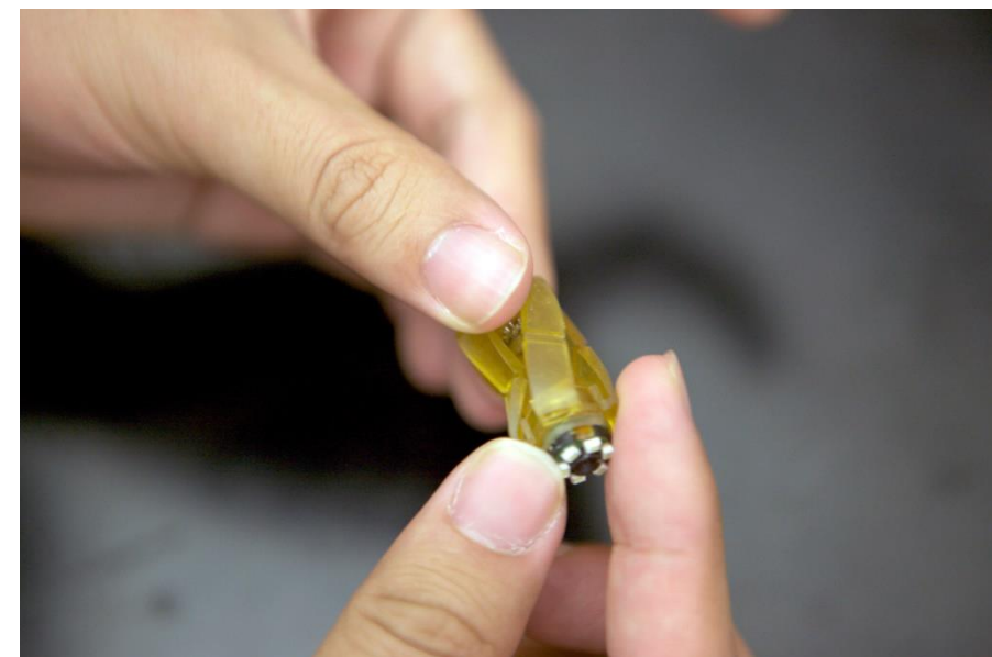
A pill-sized capsule robot capable of performing tissue biopsies and dispensing drugs
