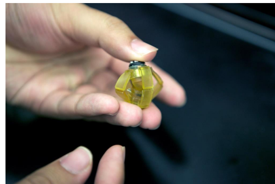
A pill-sized capsule robot capable of performing tissue biopsies and dispensing drugs
