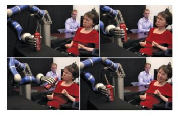
**Figure 7.7 Recordings from the brain control a robotic arm** After a stroke in this woman's midbrain cut off connections from her cortex to the spinal cord, she lost all control of her arm and leg muscles. A neural decoder connected cells in her motor primary motor cortex to a robotic arm, enabling her to pick up a coffee cup, drink from it, and put it back.
