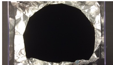
Figure 2.4: The material Vantablack composed by carbon nanotubes (Surrey NanoSystems) which, according to its manufacturers, absorbs 99.96% of incident light, on an aluminum foil.
