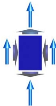
Figure 11.9.3 An imaginary box in a magnetic field (blue vectors). The short vectors indicate the directions of stresses transmitted by the field, either pressures (on the left or right faces of the box) or tensions (on the top and bottom faces of the box).
