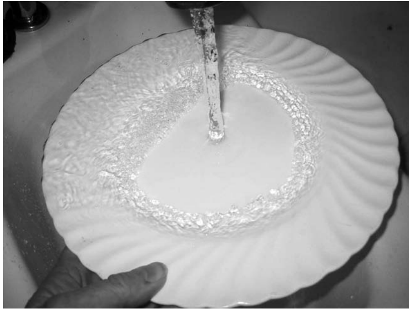
FIGURE 17.12 Hydraulic jump on a dinner plate under a kitchen tap.
