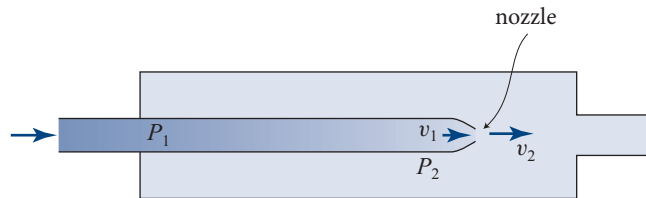
FIGURE 13.8 Schematic illustration of Joule-Kelvin cooling of a gas. Gas flows steadily through a nozzle from a chamber at high pressure P_1 to one at low pressure P_2 . The flow proceeds at constant enthalpy. Work done against attractive intermolecular forces leads to cooling. The efficiency of cooling can be enhanced by exchanging heat between the two chambers. Gases can also be liquified in this manner.
