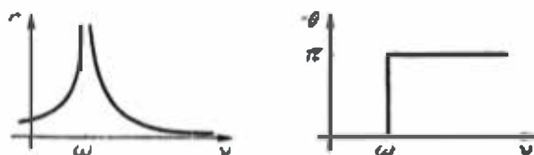
Fig. 178 The amplitude and phase of forced oscillations of a frictionless pendulum as a function of the frequency of the external force.
