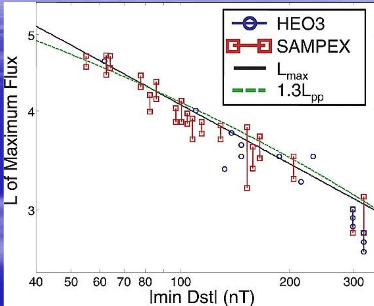
Location of the peak electron flux ( $>1.5$  MeV HEO3,  $>1$  MeV SAMPEX) as a function of minimum Dst moves to lower L
